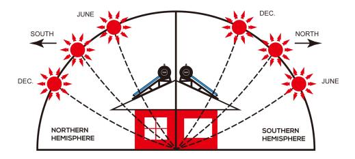
You do not have to be too careful about mounting the collector at the exact angle suggested. If your roof angle is within 10o+/- of your desired angle you can just mount the solar collector flush against the roof surface. The added trouble of adjusting the collector to a precise angle is not warranted as it will not result in a great improvement in efficiency.
