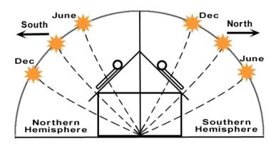
You do not have to be too careful about mounting the collector at the exact angle suggested. If your roof angle is within 10o+/- of your desired angle you can just mount the solar collector flush against the roof surface. The added trouble of adjusting the collector to a precise angle is not warranted as it will not result in a great improvement in efficiency.
