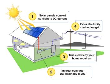
Solar modules capture the light from the sun, and through the photo-voltaic properties of the panels the light is converted into electricity. The conversion takes place within the specially fabricated semiconductor crystals comprising the cells of the solar panels.
