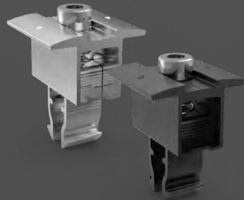
Code: PRE-EIC Premium rail mid clamp, universal for 30-45mm module, self-standing with spring, integrated with grounding pins and clip, fully pre-assembled
