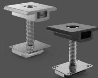
Code: ERK-EIC Standard Mid clamp, universal for 30mm-40mm framed module, fully pre-assembled with grounding clip, self standing by recessed spring.
