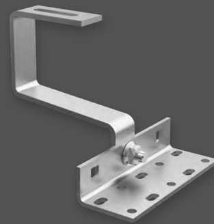
Code: ERK-TRH-T13 Spanish tile roof hook, for side mount rail Compatible with side mount rail unless an adaptor fastening kit is used Type 304 Stainless Steel Accessories: 6.3 x 80mm wooden screw, 3 pcs
