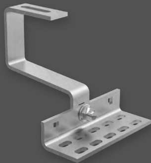
Code: ERK-TRH-T18 All tile roof hook, for bottom mount rail Compatible with side mount rail unless an adaptor fastening kit is used Type 304 Stainless Steel Accessories: 6.3 x 80mm wooden screw, 3 pcs
